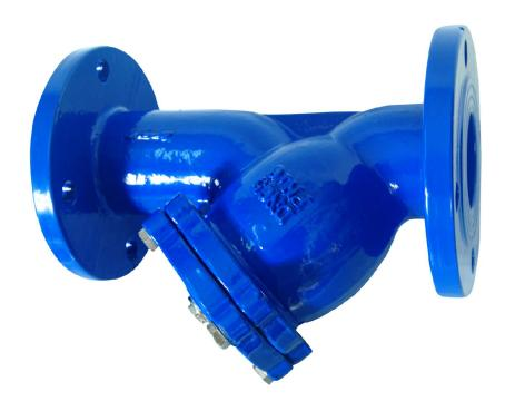
The filters F.300 are flanged Y filters, with a body made of cast iron, which are manufactured in accordance with severe product norms. They are a prerequisite for protecting pumps, valves, backflow preventers and pressure reducing valves against dirt (rust, welding parts, solids).
